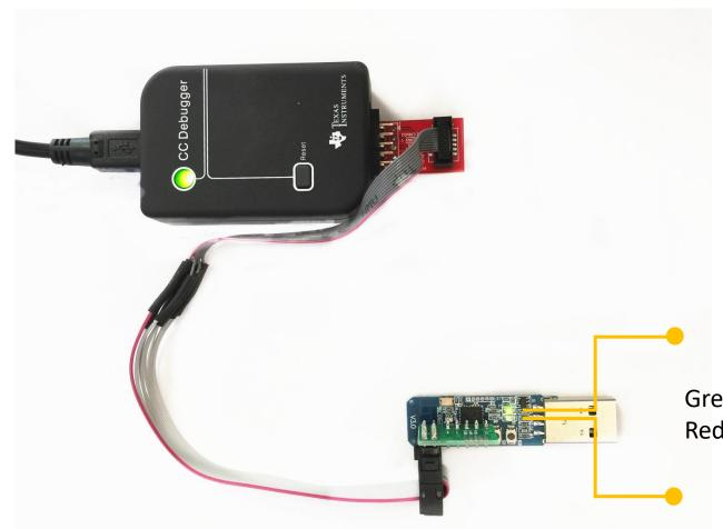
Green LED on: Configured work with Packet sniffer Red LED on: Configured work with BLE device monitor/Btool
